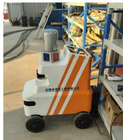
Patrol Robot at Power Grid Plant
